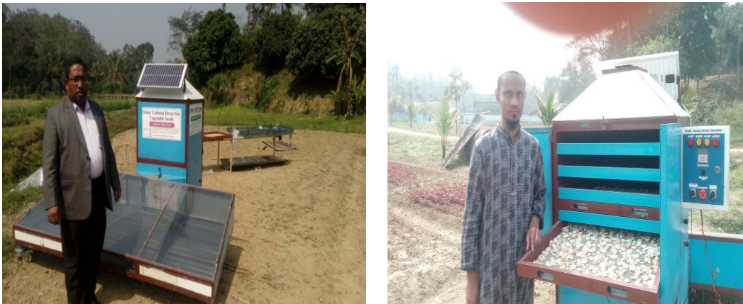
Fig. 2. Photographs showing drying of radish in BARI solar cabinet dryer
