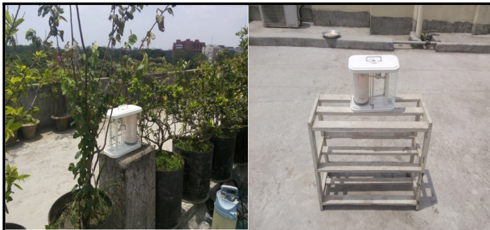
Plate 2: Taking thermal data using Thermo-hygrograph on rooftop garden and bare roof
